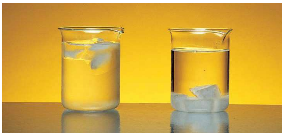
Figure 11.11 Left: Ice cubes float on water. Right: Solid benzene sinks to the bottom of liquid benzene.
